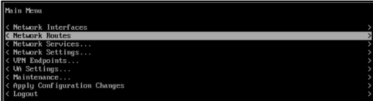
5. Use the Down Arrow to highlight **Apply Configuration Changes** and press **Enter**.
