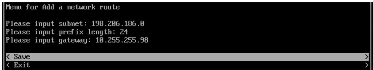
3. Enter the **Network Route Subnet**, use the Down Arrow to enter the **Prefix Length**, and the **Gateway**. Use the Down Arrow to move to **Save**, then press **Enter**.
